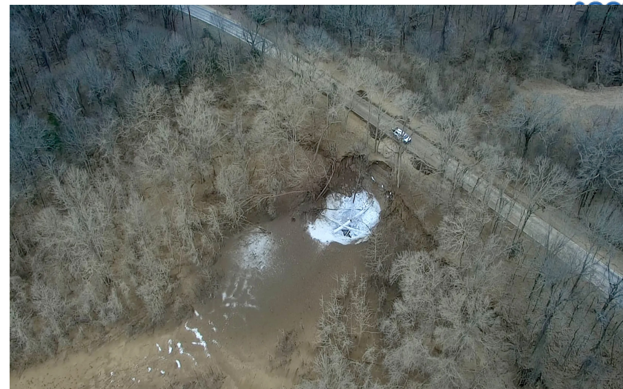
Industrial 24 inch pipe rupture, 200 barrels CO 2 , Yazoo Miss 2020. Dispersed to air in tens minutes
